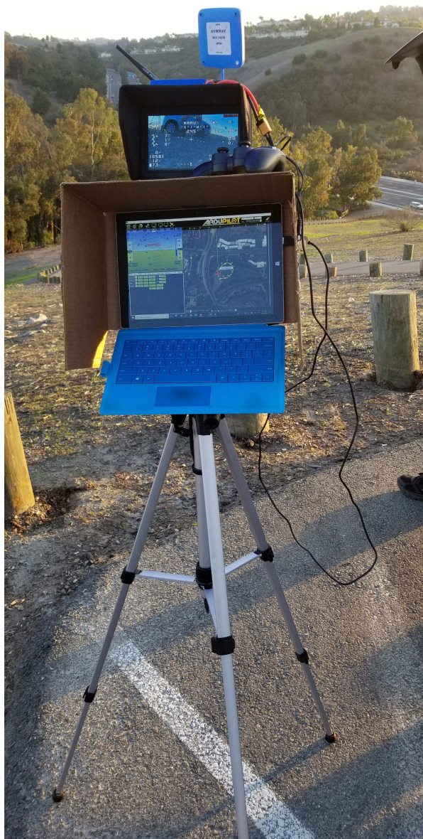
FIGURE 6. Ground control station. The Windows 10 PC runs Mission Planner to control the plane over the internet. The 7" monitor on top receives the analog video broadcast directly from the craft to the ground at 5.8 GHz.
