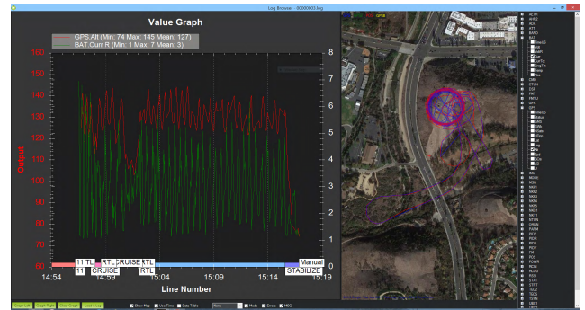
FIGURE 9. Terrain following. When circling home, MSL goes up and down to ensure AGL is constant. (Home point is on a steep sloping hill.) Also when flying in valley, MSL goes down to keep AGL constant in low valley (dip in MSL at 15:00 hours). Current high in climb; low in descent. Avg. current is 3 A. Altitude on left axis is in meters MSL. Right axis is current in A. Horizontal axis is local time (PST).
