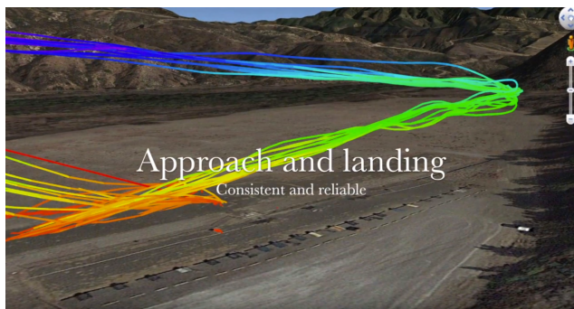
FIGURE 12. Approach and landing path of 16 separate flights shows Autoland feature to be consistent and reliable, and the landing position was consistent to within a few meters.
