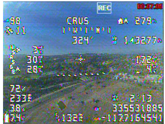
FIGURE 5. HUD. This can be customized to include, e.g. airspeed, windspeed, groundspeed, altitude, GPS coordinates, sink rate, battery voltage and current, # of GPS satellites, RSSI for radio control, flight mode, heading distance to home, etc.
