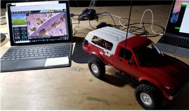
Fig. 2. Ground vehicle used for this demonstration and the laptop computer used for the remote pilot interface running Mission Planner software.
