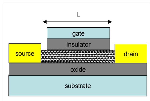
Fig. 3: Schematic of a nanotube transistor.
