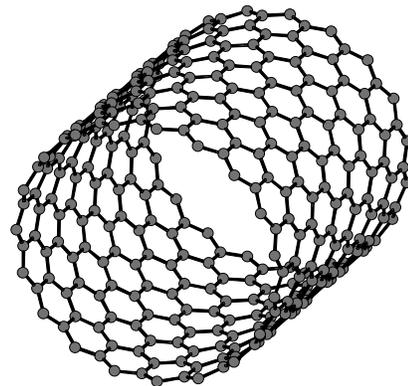
Fig. 1: Single walled carbon nanotube.
