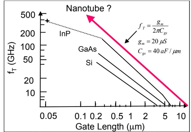
Figure 4: Predicted cutoff frequency. (From ref. 15).
