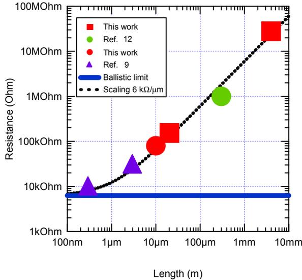
Figure 5: Resistance vs. length of a SWNT (from ref. 13).
