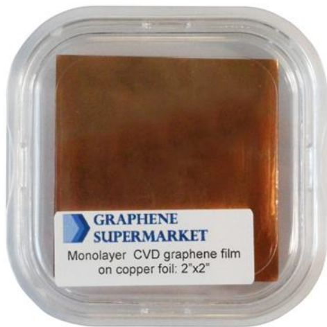
Figure 4-1. Graphene film on copper foil
