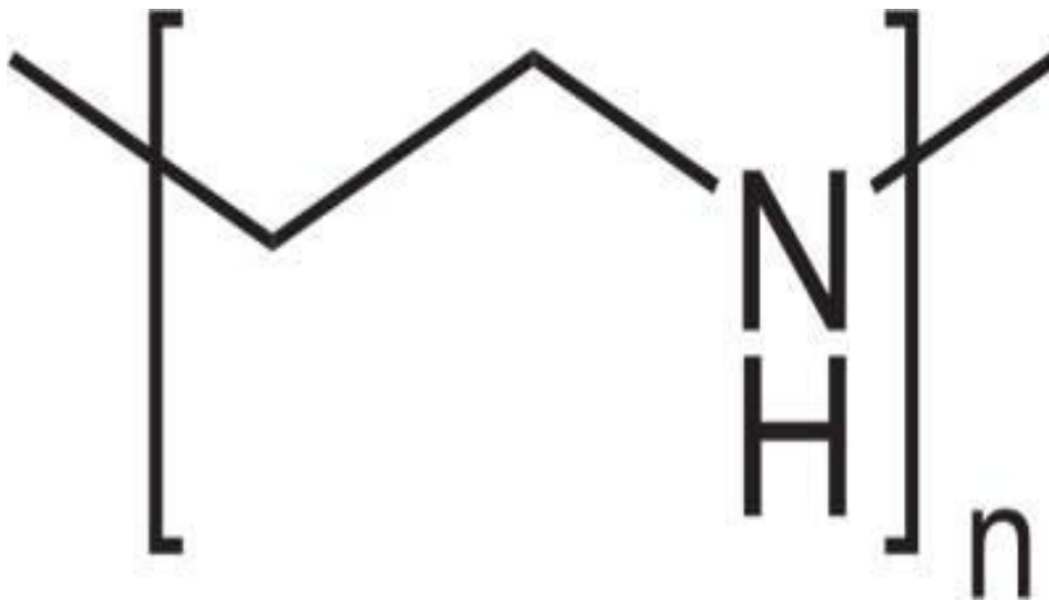
Figure 3-1. Structure of Linear Polyethyleneimine
