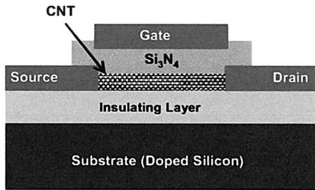
FIG. 1. Schematic cross-section view of top-gate nanotube transistor.
