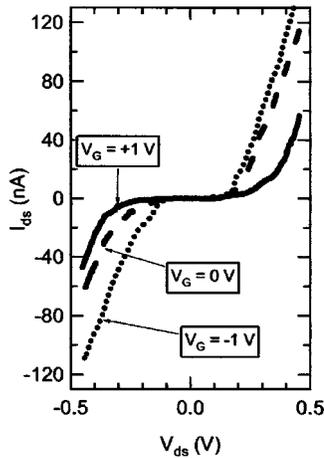
FIG. 3.  $I$ - $V$  characteristics of a top-gated CNTFET using silicon nitride gate dielectric (dielectric thickness 50 nm; gate length 10  $\mu\text{m}$ ;  $T=4$  K).
