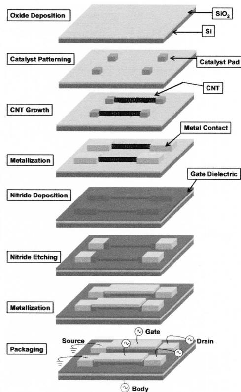
FIG. 2. Detailed processing steps (not to scale).
