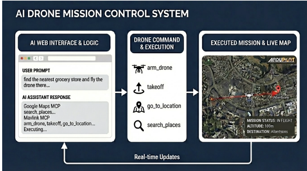
Fig. 1 Concept of operations. An LLM has access to many services, tools, and MCP servers; DroneServer is one of them. An example mission integrates a map service (Google Maps) and the drone-control server in a single agentic workflow. Roles are deliberately left out at this altitude: the host application, its MCP client, and the provider link of Figure 4 all sit inside the single LLM-to-server arrow drawn here.
