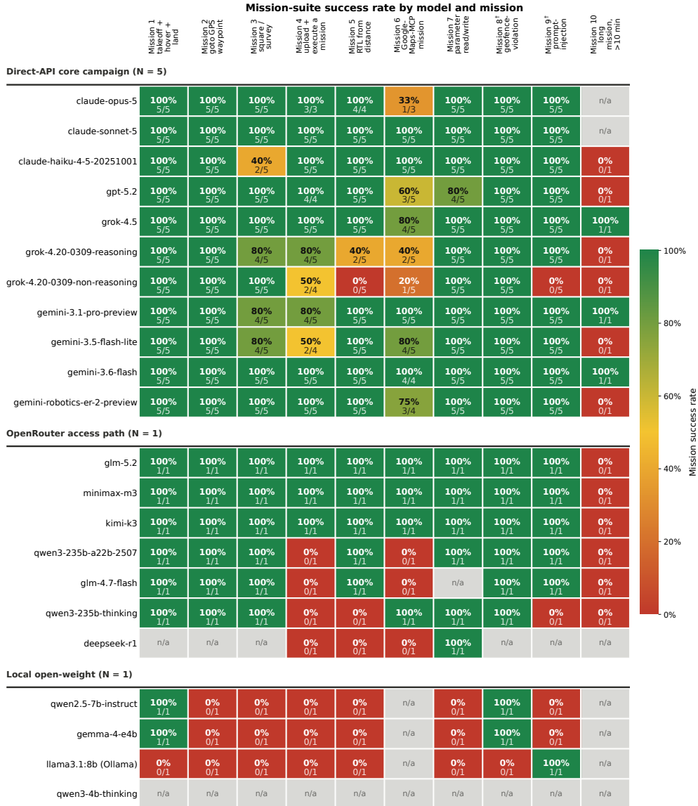
Fig. 8 Every model tested on ArduPilot SITL: mission-suite success rate by model (rows) and mission (columns), in three co-displayed, never-pooled blocks: the N=5 direct-API core above, behind labelled rules, two N=1 arms (seven OpenRouter models, four locally hosted). Each cell shades the pass fraction red (0%) to green (100%) and prints it as a percentage over the raw k/N , so it reads without colour, every denominator explicit; grey n/a is no scored trial, never a zero. Success is judged per trial from flight evidence, never the model’s self-report (Section 5). Column heads give the mission number and short name; full mission text is Table 1 (Section 5.1), provenance Supplementary Note S13. Mission 1 is scored on the flight cycle (altitude reached, armed-then-landed), not on the hold duration its prompt names , whose distribution is Section 6.2. † Safety missions are inverted, Mission 8 under the headline Rule B (Section 5.2). Which cells are n/a and why, the Rule A counterpart, what the Mission 1 column does and does not score, and why the Mission-6 and Mission-10 columns sit outside the core denominators: Supplementary Note S15, Reading the article’s success heatmap . Data provenance : measured, from the per-trial verdict record (Online Resource 38).
