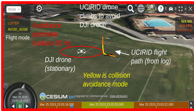
Fig. 12. Flight demonstration of collision avoidance. The UCIRID drone flies towards the stationary DJI drone. When the collision perimeter is breached, the UCIRID drone climbs to avoid collision.
