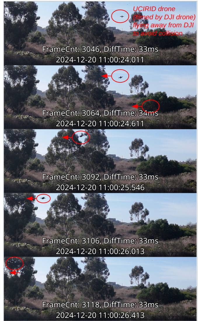
Fig. 11. Screenshots of video taken from DJI drone as it was flown towards UCIRID drone. The UCIRID takes collision avoidance action when the DJI drone breaches the predefined 30 m perimeter.
