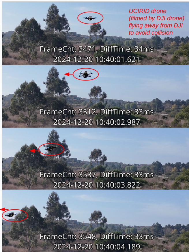
Fig. 10. Screenshots of video taken from DJI drone as it was flown towards UCIRID drone. The UCIRID takes collision avoidance action when the DJI drone breaches the predefined 10 m perimeter.
