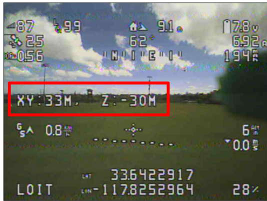
Drone detected, 33 m away (not in avoidance perimeter)
