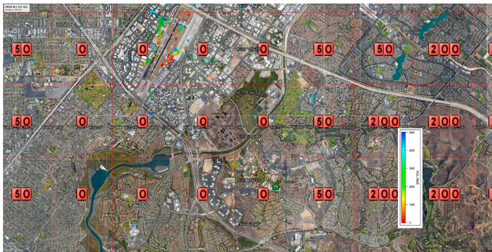
Figure 8. Helicopter-only traffic below 500' AGL near KSNV for 4/1, 5/1, and 6/1/2019. Color code: Red = 0' AGL and Blue = 500' AGL, overlaid with the SUAS facility maps. White is for aircraft with 0 AGL.
