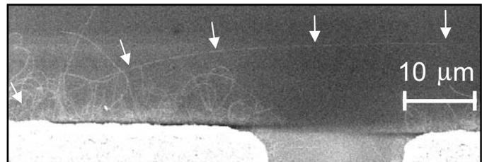
Fig. 2. SEM image of a single walled carbon nanotube. Length is 60  $\mu\text{m}$ .
