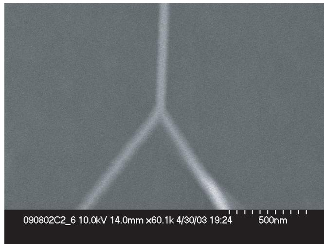
Fig. 4. High resolution SEM image of Y-junction.
