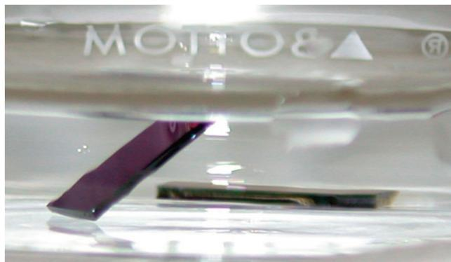
**Figure 3.** SWNT sample on a SiO<sub>2</sub> wafer suspended in water with the edge barely exposed to air while a SiO<sub>2</sub> wafer with no nanotubes sinks to the bottom of the glass container before half of its area is submerged in the water.
