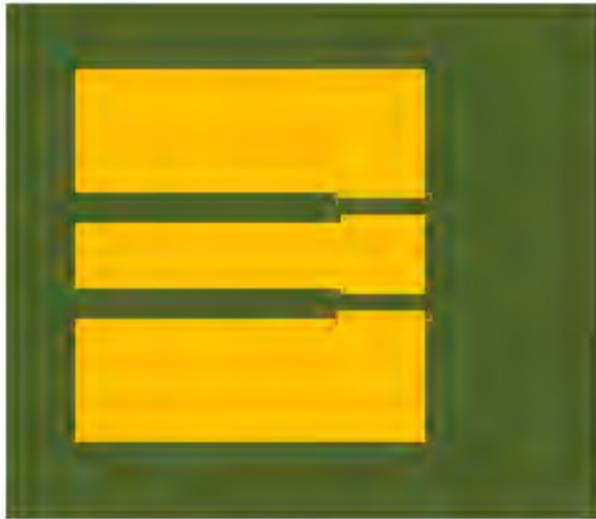
1) Coplanar Waveguide on wafers
