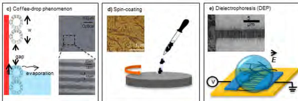
Figure 3.2. Deposition techniques [3]. Random deposition methods: a) Gravure printing using carbon nanotube ink [48]. b) Inkjet printing of nanotube ink [70]. Semi-aligned networks: c) Coffee-ring method using the surface friction for depositing nanotube strips [69]. d) Spin coating the nanotube ink resulting in radial alignment of nanotubes [46, 47]. e) Dielectrophoresis deposition which usually leads to preferential deposition of metallic tubes over semiconducting tubes [75, 76].
